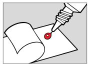
6 Gently squeeze a small drop of Control solution onto the inside of the foil you saved in Step 3.
